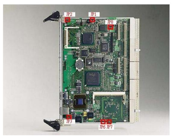
Figure 1-2: MIC-3368 jumper and connector locations.
